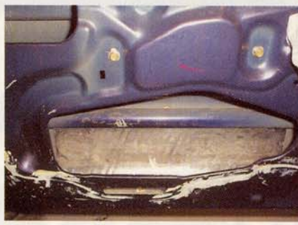
7. We also applied a larger piece in the rear section of the door to help gain some much needed mid-bass.
