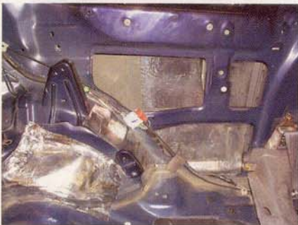
10. We applied the Brown Bread to the outer quarter panel skin, the inner fenderwell, and the strut tower itself. This made a huge difference considering Honda all but forgot about these very noisy areas.
