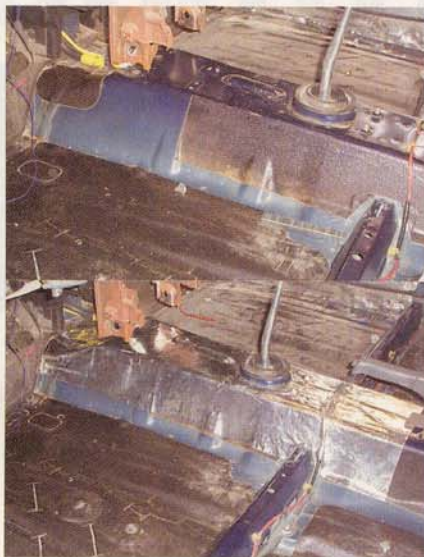
8. The tranny tunnel is another trouble area. Rather than remove the factory material, we laid the Brown Bread over the top of it and doubled it up.
