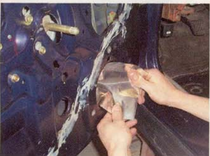
6. After we cut our pieces, we removed the backing to expose the adhesive and applied it to the outer door skin. To our surprise, we needed no heat to activate the glue. This stuff is really sticky.
