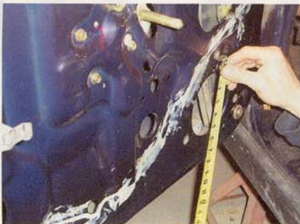
4. The outer door skin seemed like a good place to start, so we made a few measurements.
