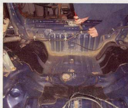
11. When the subs were turned up, the whole back of this Civic rattled like crazy. We couldn't deal and started by removing the clips that held the wiring harness in place. To help keep track of the holes, make a template out of paper (we used the backing off the Brown Bread) and poke out the holes with a screwdriver.
